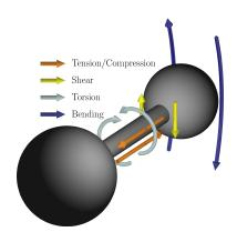
Figure 3.7: Diagram illustrating the forces and moments between particles bonded via rotational elastic-brittle bonds
