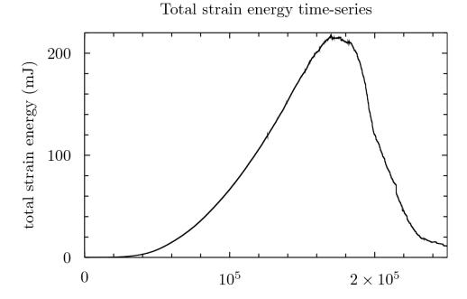
Figure 3.10: Time-series of total strain energy stored in bonds during a uniaxial compression simulation (from rot\_compress.py)
