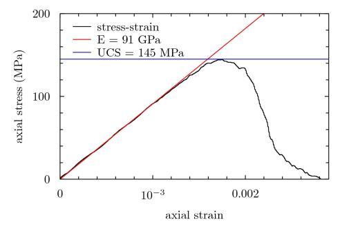
Figure 3.9: Stress-Strain curve obtained from a uniaxial compression simulation (from rot\_compress.py)
