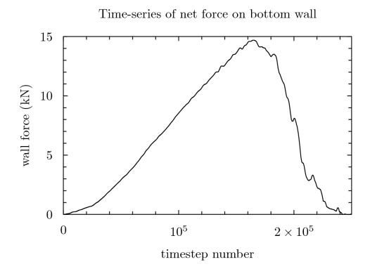
Figure 3.12: Time-series of net wall force during a uniaxial compression simulation (from rot\_compress.py)
