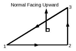
Figure 3.5: Specification of mesh nodes for wall normals
