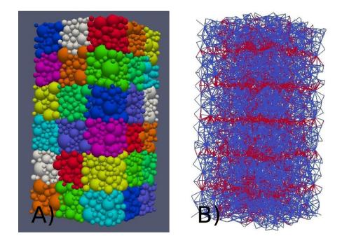
Figure 4.3: Images (generated with Paraview) of a box with clustered particles generated by the script cluster\_box.py described in section 4.5. Panel A) shows the particles colored by particle tag. To enhance the visual contrast between neighboring clusters colors are set using particle tag modulo 10. Panel B) shows the bonds in this model. Intra-cluster bonds (bond tag 0) are shown in blue and tags between clusters (bond tag 1) in red.
