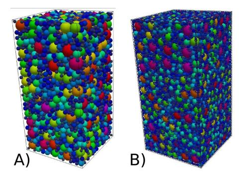
Figure 4.2: Images (generated with Paraview) of a box with particles fitted to the box faces generated by the script smooth\_box.py described in section 4.3. The model in A) uses particle radii between 0.2 and 1.0, the model in B) uses particle radii between 0.05 and 1.0.
